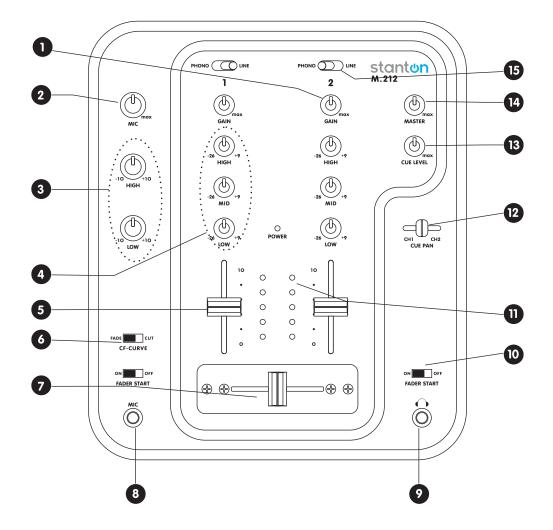
1. Channel Gain - Adjusts the pre-fader volume for cleaner sound. Reduce the channel gain if you notice the level indicators flashing red.
